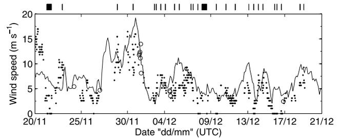
**Figure 2.** Wind speed observations in the Amundsen Gulf during the sampling period. NCEP-NARR reanalysis (solid curve), CCGS Amundsen navigation anemometer reported in the science log book during sampling operations (black dots), and meteorological science station aboard the CCGS Amundsen (circles). The black lines at the top indicate the sampling periods reported here.
