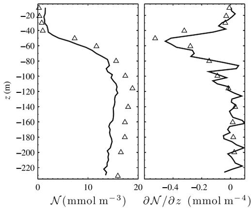
**Figure 3.** Example of (left) a typical nitrate profile and (right) its gradient (3 December 2007). The triangles represent measurements from laboratory analyses of bottled water samples and the solid lines represent the 4-m scale calibrated Isus-V3 sensor measurements.
