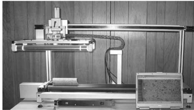
**Figure 3** Smartcube smartCIS camera image scanner. In this figure, the digital image of a whole rock core was acquired, unrolled and displayed on the companion laptop. Image modified with permission from <http://www.smartcube.de/indexeng.htm>
