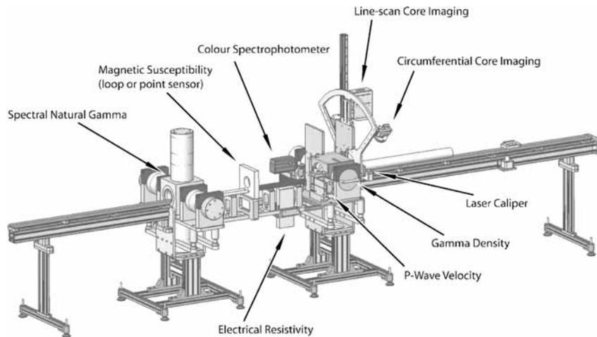
**Figure 1** Schematic diagram of a GEOTEK Multisensor Core Logger, MSCL (suitable for both whole or split lined sediment cores and unlined rock cores), illustrating the range of sensor systems available (see text for details). The specific suite of sensors on any given MSCL depends on user requirements and may include a digital X-ray imaging system (not shown).
