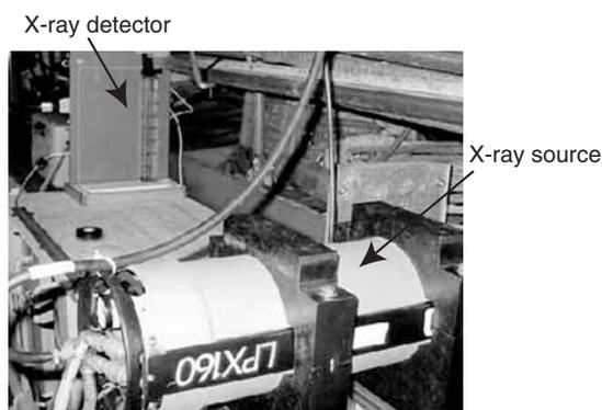
**Figure 5** Oregon State University (OSU) portable shipboard digital X-ray system onboard the *R/V Garcia del Cid*. The X-ray source and detector are shown.
