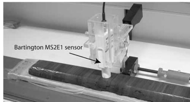
**Figure 2** TAMISCAN-TS1 point-source magnetic susceptibility track. The system uses a Bartington MS2E1 sensor. A split core covered by a plastic sheet is being measured.
