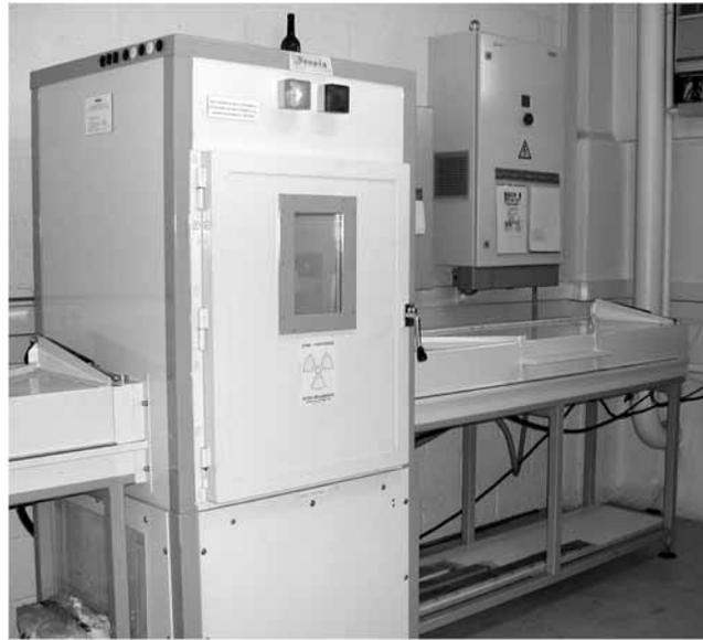
**Figure 4** Photograph of the complete SCOPIX system showing the X-ray lead-protected box and the two sleeves on each side.
